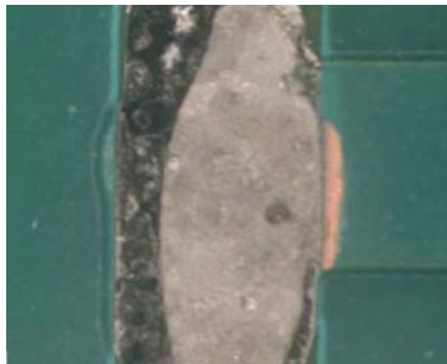
Figure 5: Issues with assembled PWB: dewetting and black residues.
