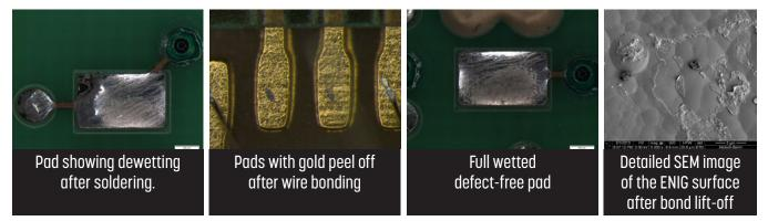
Figure 2: Exemplary pictures of failure modes of ENIG finishes in soldering and bonding.
