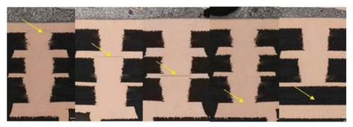
Microvia "partial" fractures found throughout stacked electroless Cu interfaces, as well as within the laminate resin, which indicates CTE-z stresses essentially the same at all levels.
