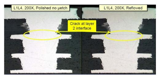
Figure 2: Two microvia stacked constructions with the typical microsection on the left, where the problem is invisible, compared with after reflowing, where it is almost invisible. (Source: Motorola Solutions)
