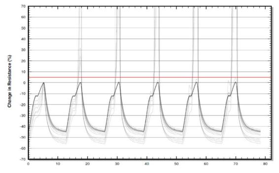
Figure 18: Resistance during the reflow of Net1 (notice that all coupons pass the first cycle).
