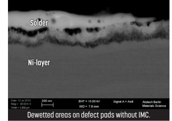
Figure 3: Exemplary SEM images of defect pads in a cross-section.
