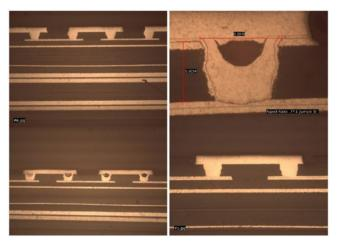
Figure 15: Example of WMI failure caught by OM testing.
