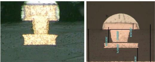
Figure 20: Remake with correct via and dielectric.
