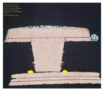
Figure 1: Older microvia failure due to contamination on the landing pad.
