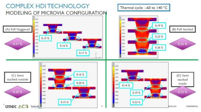
Figure 6: IMEC and ESA test simulations with actual builds and thermal stresses.
