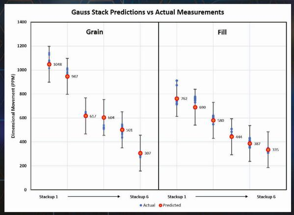
A study of 6 different stackups (using 4 different materials) was conducted to verify our results with those of actual manufactured PCBs. Above, we have plotted the Gauss Stack predictions for dimensional movement against the actual measured movement on built boards. As these data demonstrate, the predictions from Gauss Stack are very accurate.
