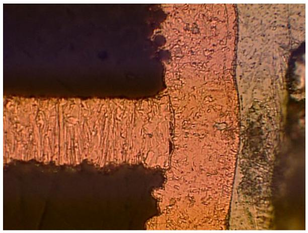
Figure 2: Type 1 ICD.
