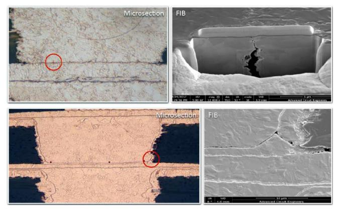
Figure 7: The older methods fail at detecting weak microvia defects.
