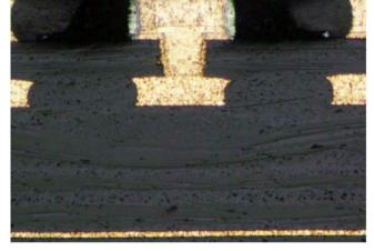
Figure 16: A microvia at 0.005" with an aspect ratio of 1:1 and a dielectric target of 0.0045".
