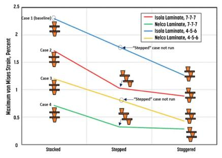
Figure 7: The effect of varying microvia configurations shows stacked as the most strained and staggered as the least strained. (Source: Raytheon)
