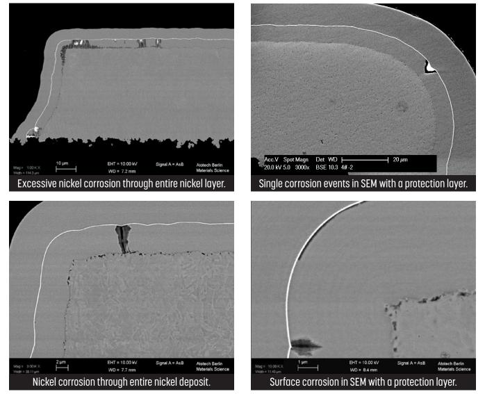
Figure 1: Exemplary pictures of different types of ENIG corrosion.
