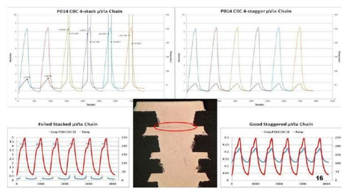
Figure 3: Two sets of three-level microvias, left-stacked, thermal cycled to reflow temps, opened, and then closed when cooled. Right-staggered and no-open/resealed connections. (Source: Motorola Solutions)
