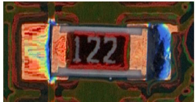
Figure 17: Bad solder joint sample.
