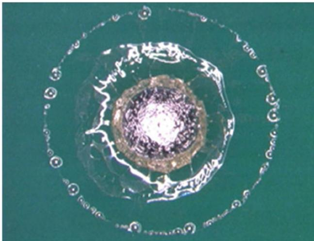
Figure 6: Random solder balls due to paste deposited on solder mask.
