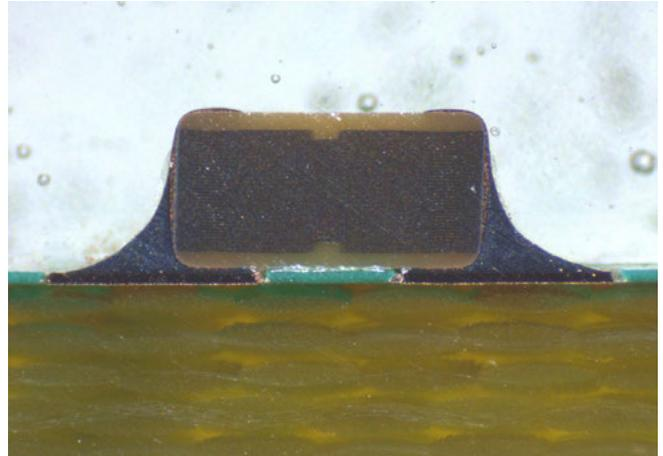
Figure 13: Solder joint profile.
