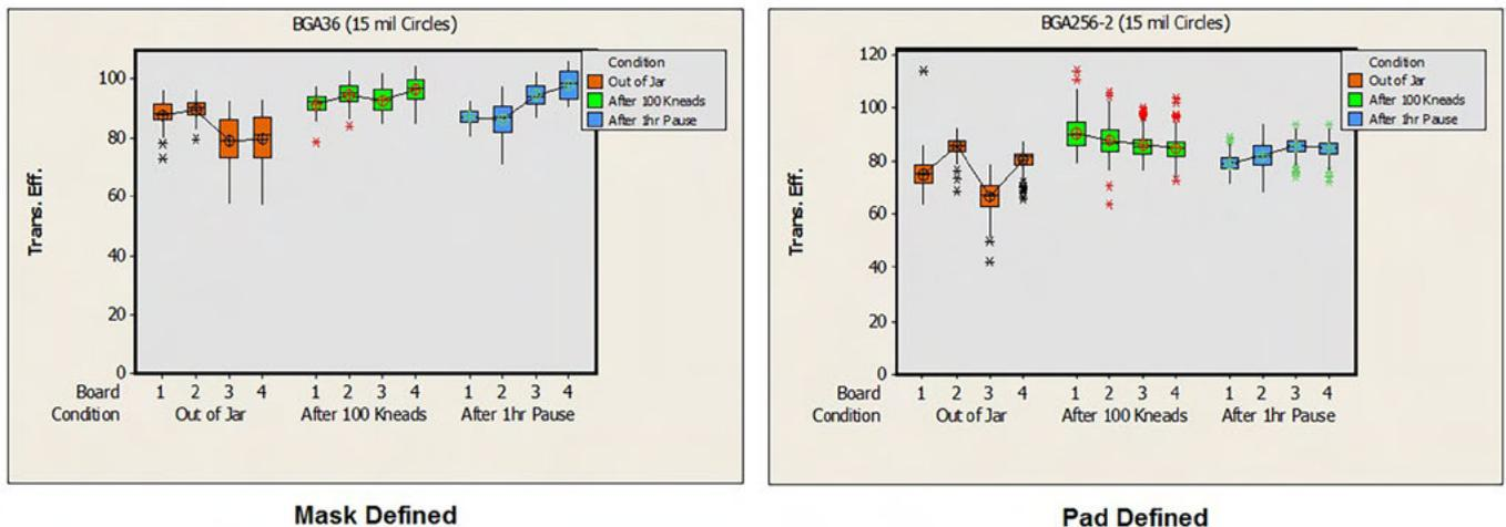
Figure 1: A print volume histogram of two sets of 15 mil (380 micron) diameter circular features on the same board.
