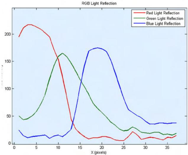
Figure 7: The observed RGB color variation along the solder joint profile.
