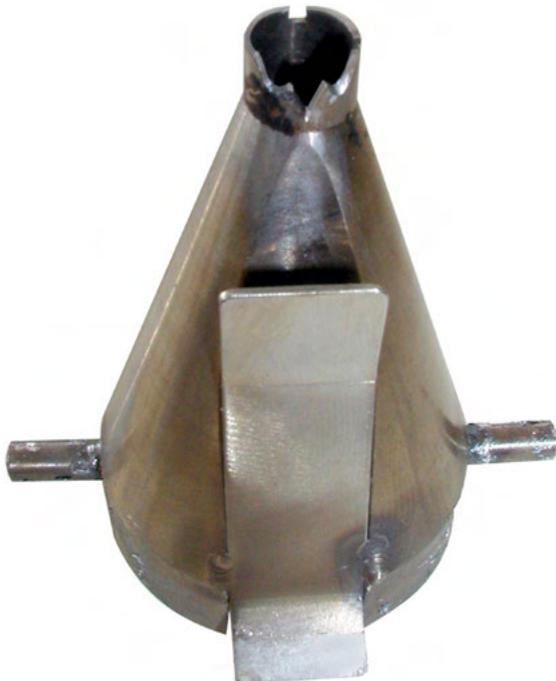
Figure 1: Example of typical jet nozzle.
