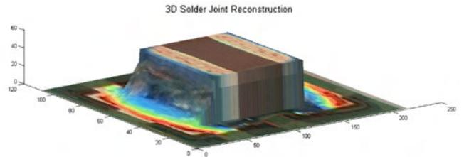
Figure 14: 3D-SJR applied over the ceramic capacitor.
