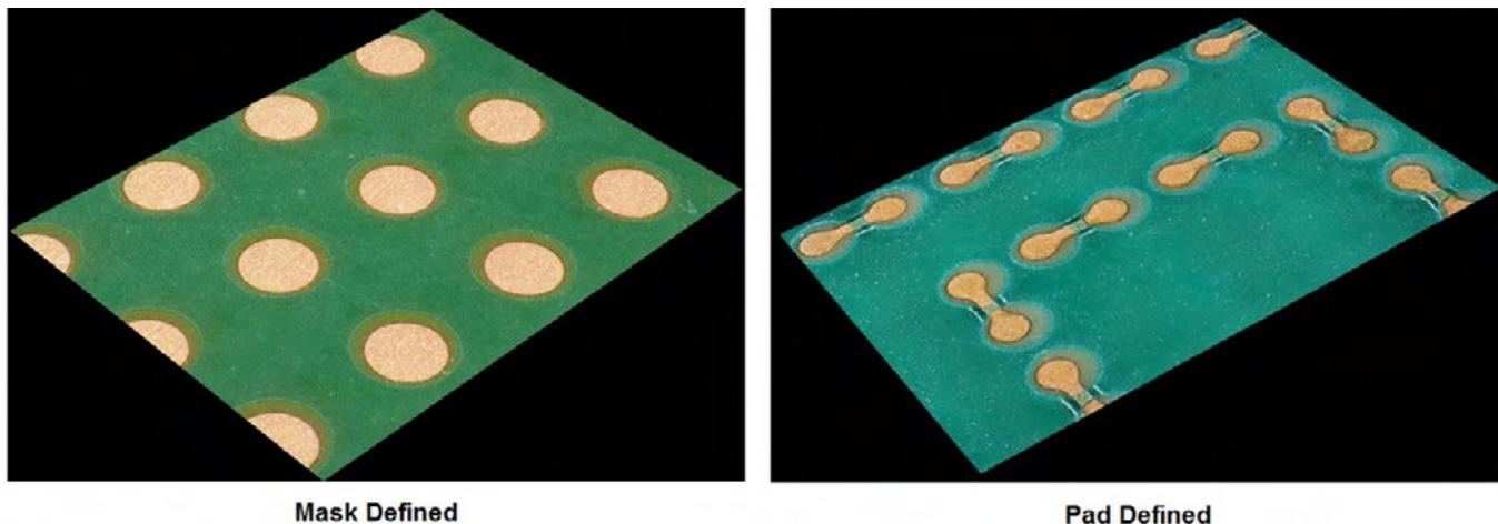
Figure 2: 3D photos of both mask defined and pad defined circles of the same size.
