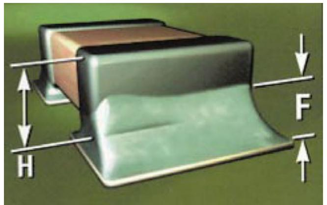
Figure 11: Solder joint height<sup>[9]</sup>.
