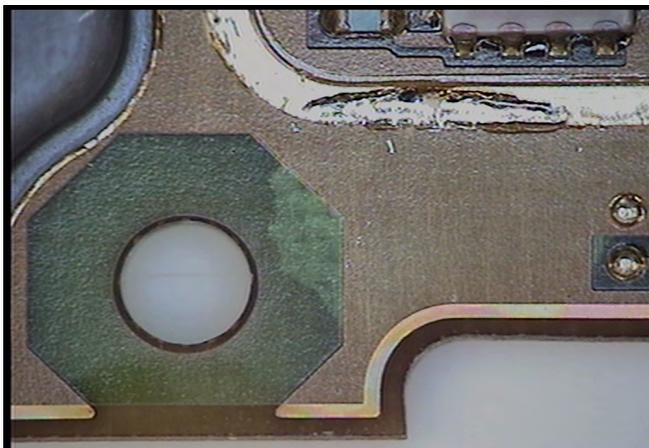
Figure 2: Resultant delamination near rework area on PCB.
