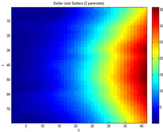
Figure 9: Solder joint height variation.
