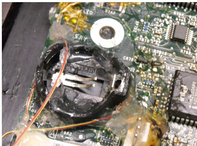
Figure 1: Shielding gel protects heat-sensitive components in areas close to rework.
