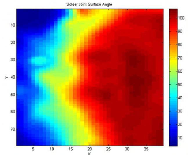
Figure 8: Surface angles along the solder joint.
