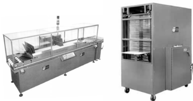
Figure 5: Two typical accumulators for conveyor processes.
