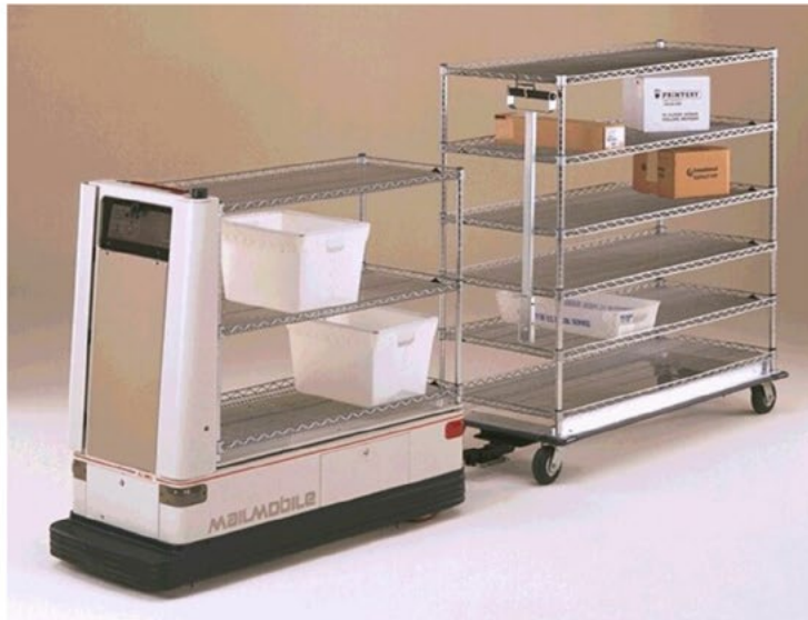
Figure 8: A few of the many AGVs commercially available today. They can follow painted stripes on the floor, be wireless guided or use GPS location.
