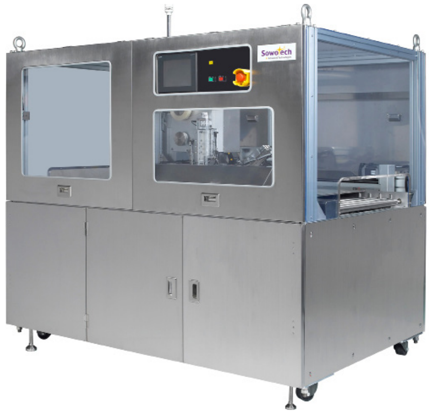
Automatic mylar peeler is needed prior to DES (from Sowotech).
