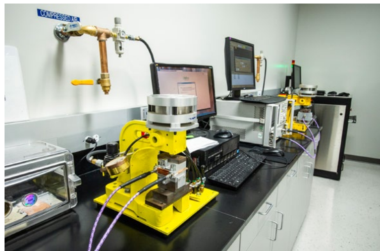
Example of one type of equipment used for measuring Dk/Df of base materials.
