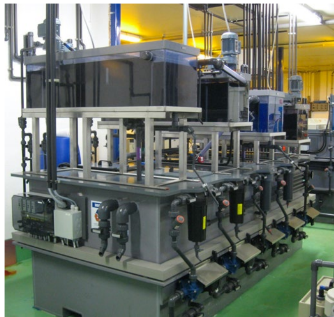
Figure 5: An actual LLE mixer-separator in operation at a working PCB fabricator. (Source: Sigma Engineering)
