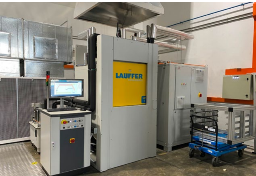
SG Lab Press—new R&D scale press system in Isola's Singapore lab.
