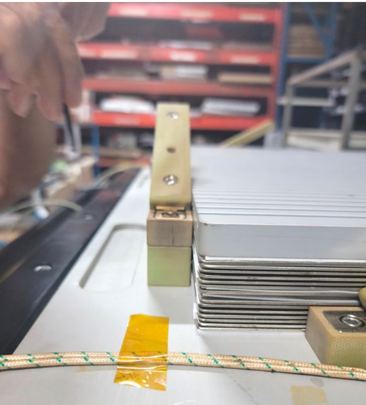
Close up view of the Indubond press in action.
