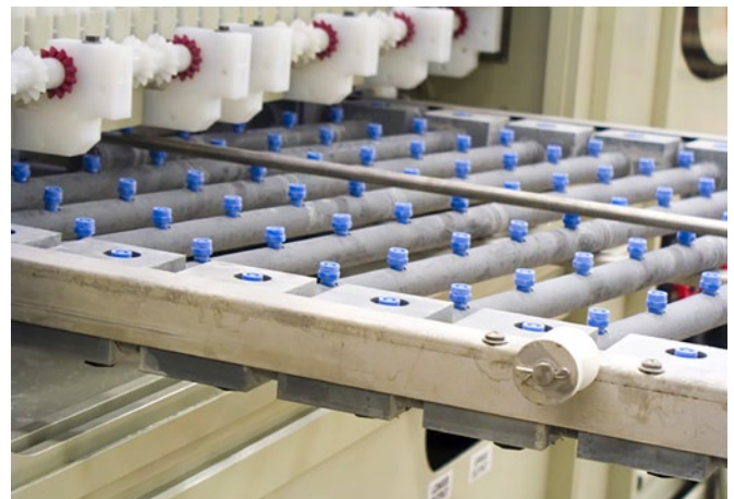
Figure 2: A lower spray rack being removed from an etcher to check nozzle condition.
