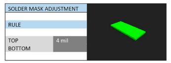
Figure 3: Setting the solder mask clearance values of your design tool.
