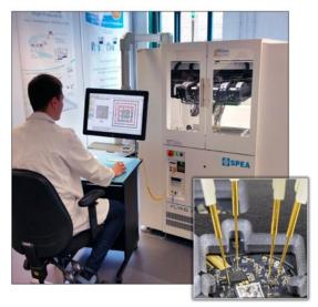
Figure 3: Flying probe test system for providing maximum access. (Source: SPEA Test Systems)
