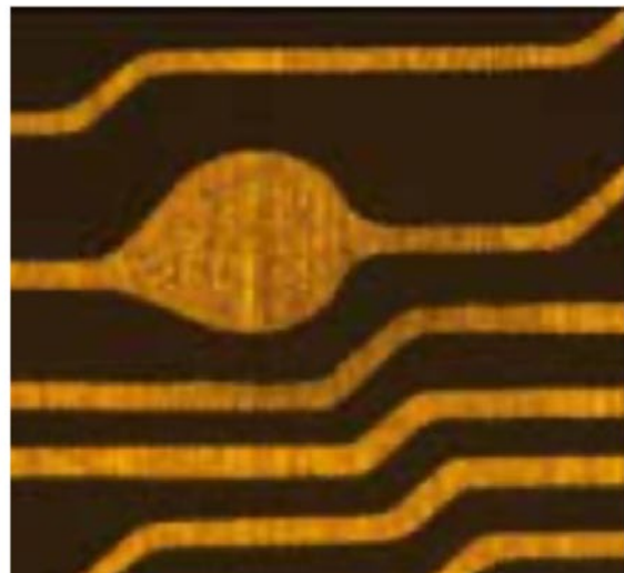
Figure 1: 3D laser ablation enables precise reshaping and elimination of excessive solder.
