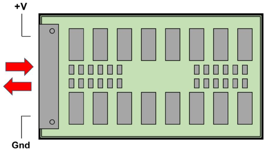
Figure 1: Functional circuit test access using I/O connector.
