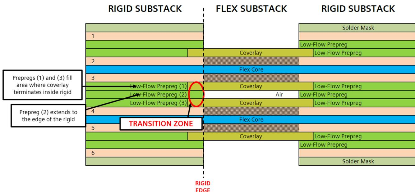
Figure 7.2: Coverlays from flex substacks are nested within a transition zone in the rigid substack.
