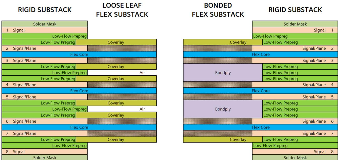
Figure 7.3: Loose-leaf designs are most flexible for 90- and 180-degree bends. They are the simplest to manufacture but not recommended for impedance control. Bonded is less flexible, thus requiring a more generous bend radius.
