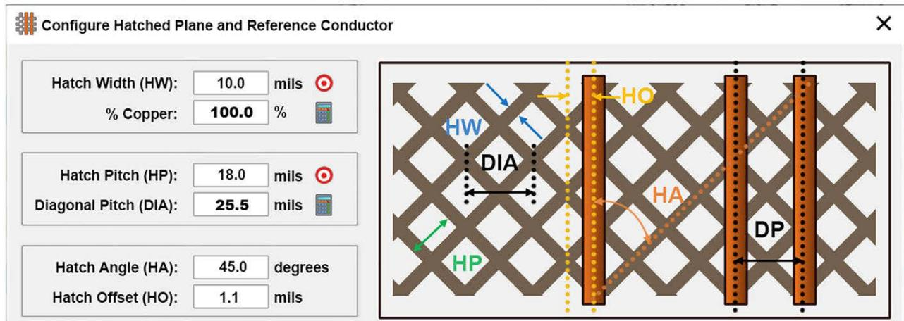
Figure 7.5: In this example, the hatch pitch is 18. The diagonal pitch is 25.5. Hatch angle is 45 degrees, and the hatch offset is 1.1 mils, but ideally would be zero. (Image from Z-planner Enterprise.)
