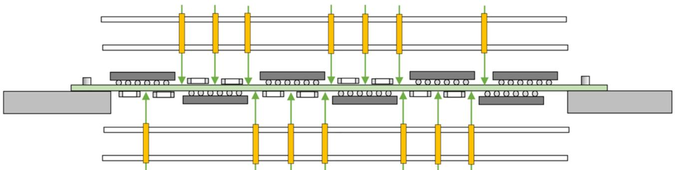
Figure 3: In-circuit test fixture with two-sided probe access.
