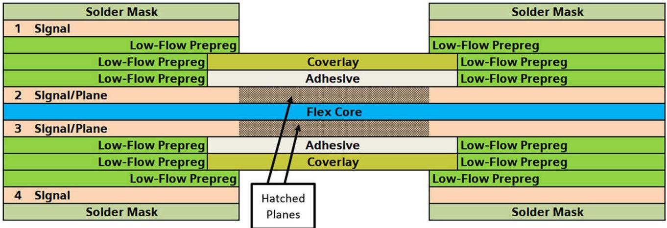
Figure 7.4: A 4-2-4 stackup design. Although this example has an even number of layers, rigid-flex stackups can also have an odd number of layers, somewhat unique to rigid-flex designs.
