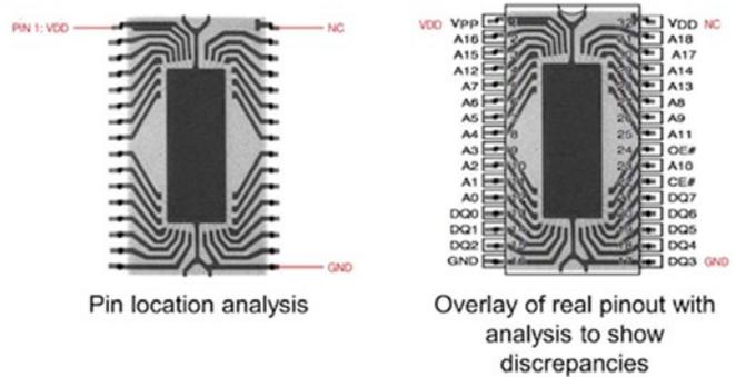
Figure 4: Example of missing wire bonds.
