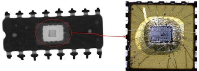
Figure 5: A wire bond ball and loop inside a package should sound alarm bells.
