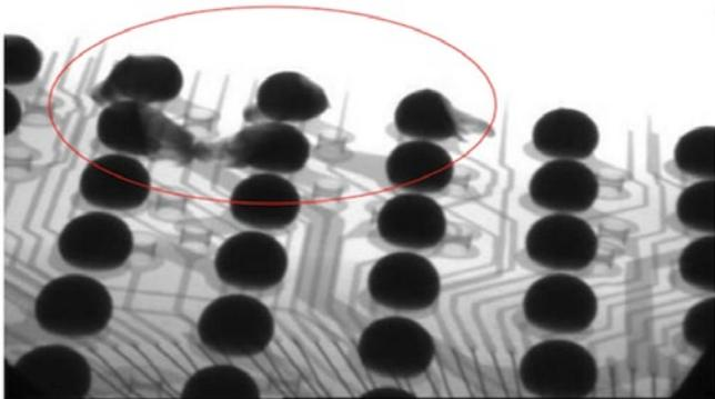
Figure 7: An example of a bare component with a large amount of voiding.
