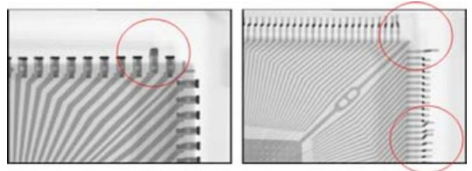
Figure 9: Components with anomalous die attach voiding.
