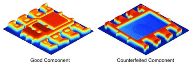
Figure 1: 3D renderings show the entirely different structures of two devices from the same lot.
