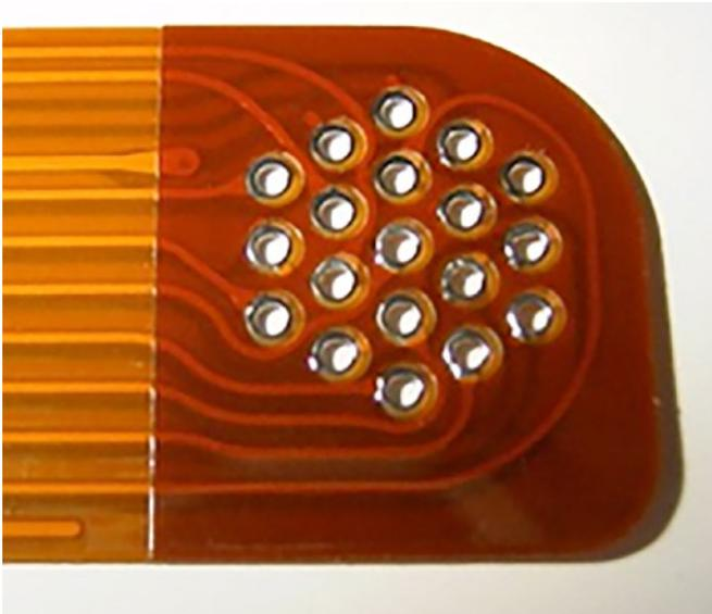
Figure 2: A 5-mil double-sided, thick cover coat used as a stiffener on a 1-mil very flexible circuit.
