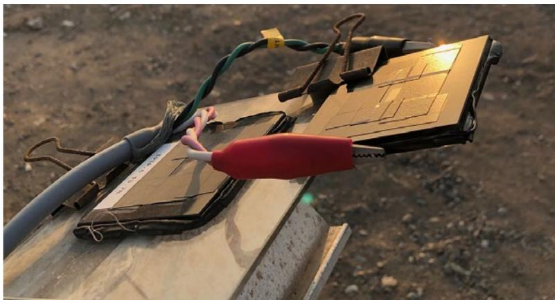
A bifacial perovskite/silicon solar cell prototype is field-tested at King Abdullah University of Science and Technology in Saudi Arabia. (photo courtesy of Michele De Bastiani)
