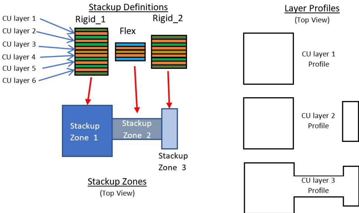
Figure 1: Stackup groups assigned to stackup zones and layer profiles are provided in IPC-2581 Revision C.
