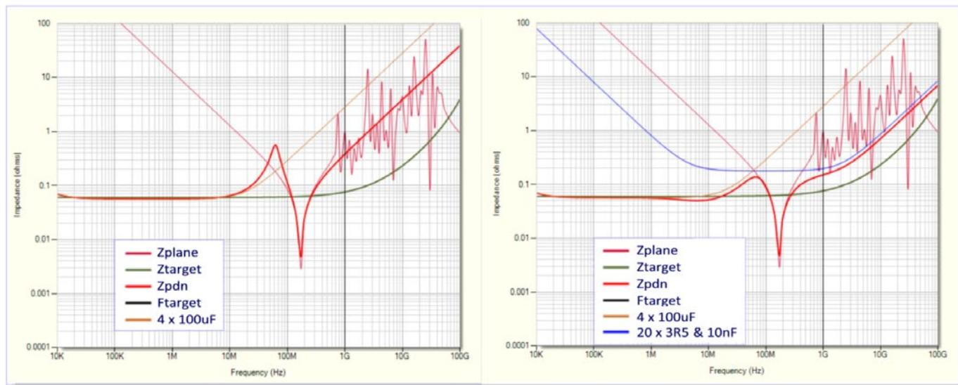
Figure 2:  $Z_{pdn}$  with 4x100uF (left),  $Z_{pdn}$  with added RC damping (right). (Source: iCD PDN Planner)
