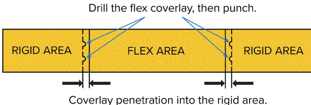
Figure 1: Define the coverlay by using drilling and punching.
