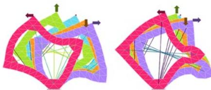
A simulated soft robot controlled to reach the same target (red dot) while acting either soft (left) or stiff (right).
