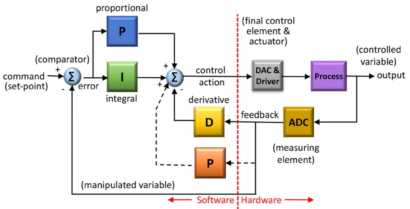
Figure 1: Basic PID controller. (Source: Tim Wescott [1])
