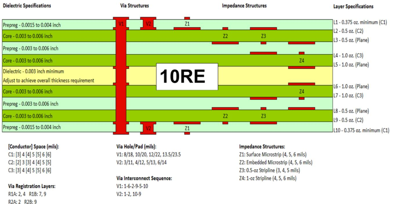
Figure 1: 10R-E panel stackup and via/trace structures.
