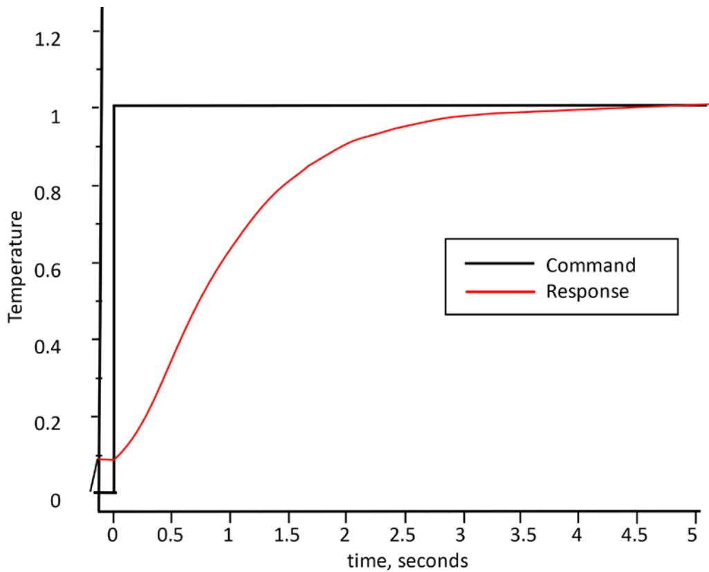
Figure 4: On-off control response <sup>[1]</sup>.
