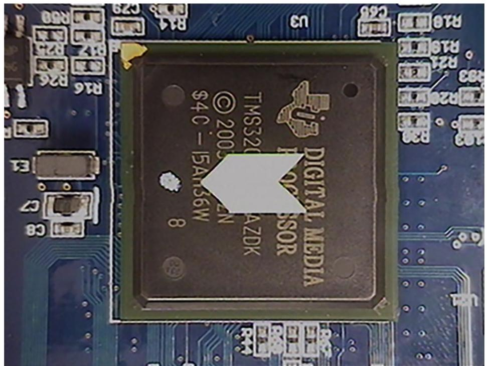
Figure 2: Re-balled BGA marking after salvaging.
