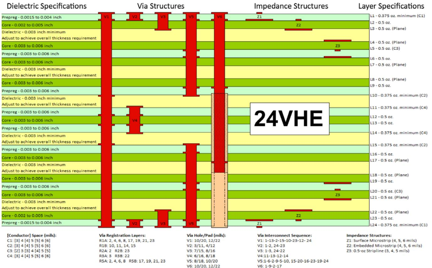
Figure 3: 24VH-E panel stackup and via/trace structures.
