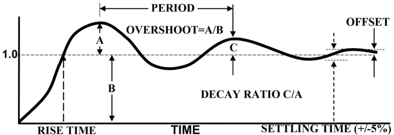
Figure 3: Characteristics of common controller responses.
