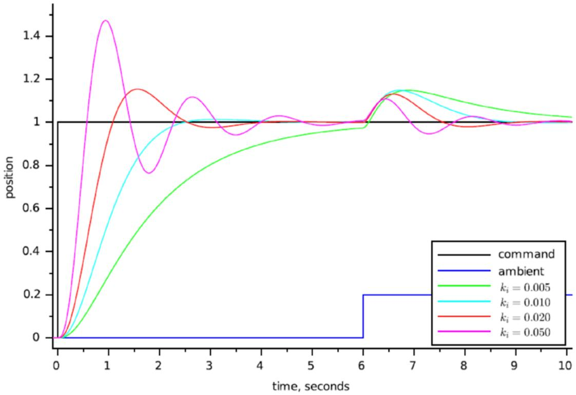
Figure 6: Integral control response. Motor and gear with proportional feedback position vs. time <sup>[1]</sup>.
