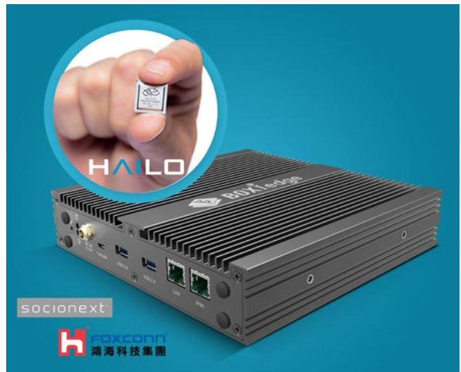
Figure 2: The aim of the BOXiedge is to be able to process multiple video streams and different applications using a single Hailo-8 device.
