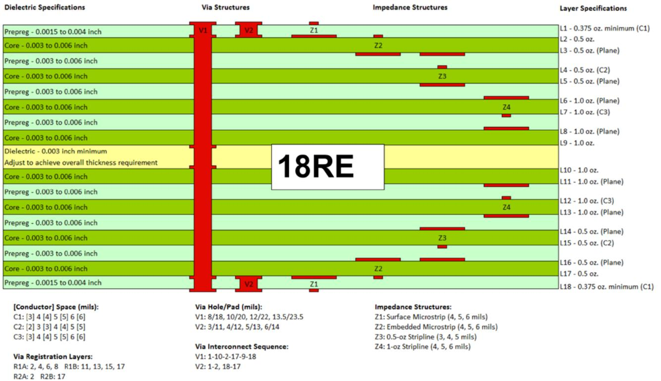
Figure 2: 18R-E panel stackup and via/trace structures.
