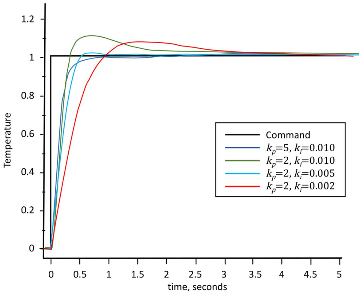
Figure 8: Response of the precision actuator system with PID control. This system settles in less than half a second compared to multiple seconds for other systems<sup>[1]</sup>.
