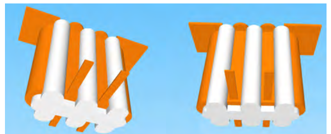
Figure 1: The basic VeCS element shown from the bottom side using two traces and a power connection at the far end of the slot. Terms for the wide structures are cross route and bottom route.
