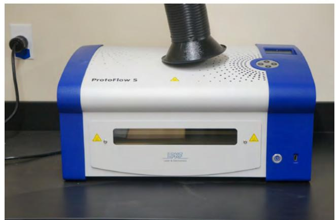
LPKF benchtop convection oven used at GFU for lead-free reflow soldering.
