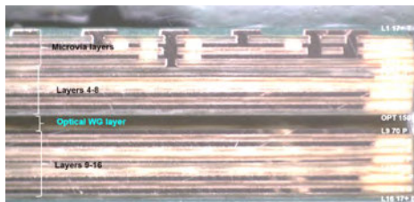
Figure 4: PhoxDem09.04MPX – 18L+2 opt embedded WG layers.
