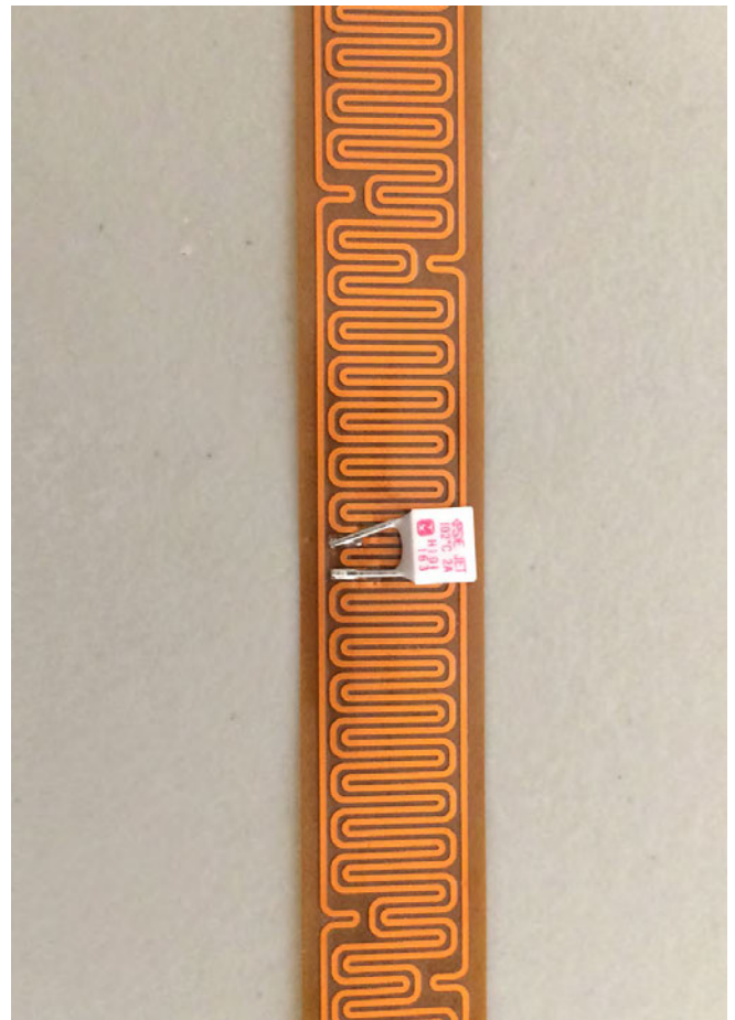
Figure 4: Thermal cut-off device on a flexible heater.
