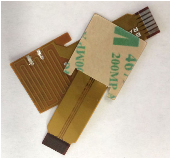
Figure 5: ZIF tail on a flexible heater.
