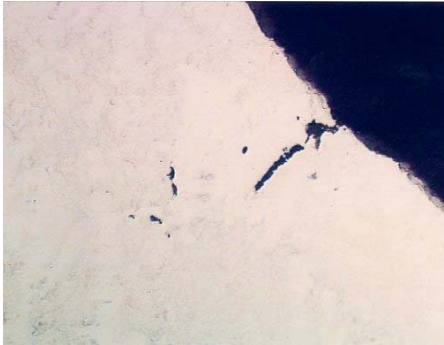
Fig. 10. Crack in “lead-free” through-hole joint
